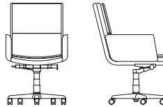
587-5 Medium Back, Swivel/Knee Tilt, Casters, Pneumatic Height Adjustment, Fully Upholstered Closed Arm W 25" D 29" H 38-43" SH 18-23" AH 26-31"
