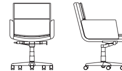
580-5 Low Back, Swivel/Knee Tilt, Casters, Pneumatic Height Adjustment, Fully Upholstered Closed Arm W 25" D 28" H 33-38" SH 18-23" AH 26-31"
